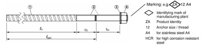
Figure A10: Rebar Ø8, Ø10, Ø12, Ø14, Ø16, Ø20, Ø22, Ø24, Ø25, Ø28, Ø32
