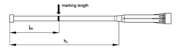
On the static mixer and the extension pipe the mortar filling mark  $l_m$  and the drill hole depth  $h_1$  must be marked with an adhesive tape or text marker. Rough estimate:  $l_m = \frac{1}{3} \cdot h_1$  Fill in the mortar as long until the filling mark  $l_m$  will be visible.
