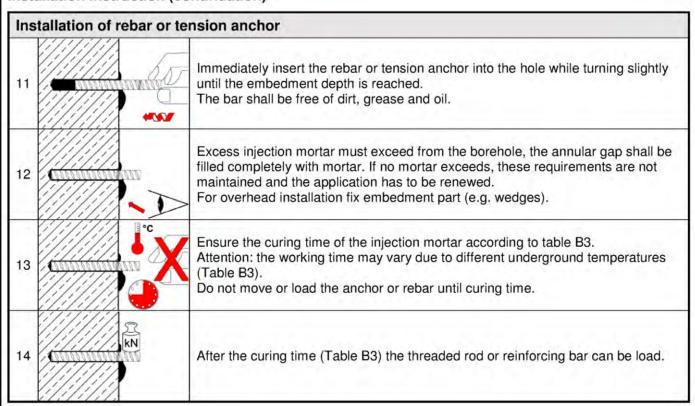
Injection System VHM for rebar connections
