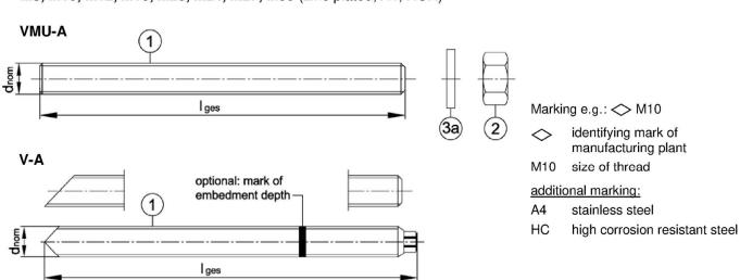
Threaded rod VM-A (material sold by the meter, to be cut at the required length) M8, M10, M12, M16, M20, M24, M27, M30 (zinc plated, A2, A4, HCR)
